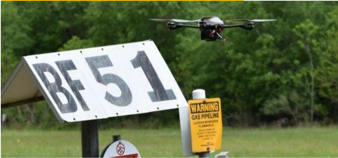
IMAGE 2017: RMLD UAV DRONE developed by Heath Consultants Inc., Princeton University & Physical Sciences Inc. - an autonomous, natural gas leak detecting, locating, quantifying and reporting system.
